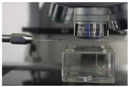
Fig. 10: Thin glass microneedles mounted on micromanipulators and used under an optical microscope to manipulate Stardust samples.
