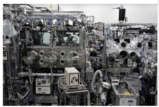
Fig. 2: Specially designed clean chambers used for handling samples and also for storage.
