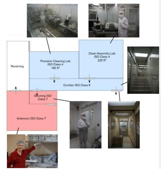
Fig. 6: Schematic viewgraph of the clean rooms of the Genesis Facility. Pictures showing (from top, clockwise): (i) Aurore Hutzler in the Precision Cleaning Lab, (ii) Judith Allton in the Clean Assembly Lab, in front of a FT-IR, (iii) the corridor in the cleaner part of the lab, (iv) the emergency exit from outside, (v) Aurore Hutzler in the garment room, adjusting an ISO 4 gown, and (vi) Judith Allton in the Anteroom, wearing only minimal protection.
